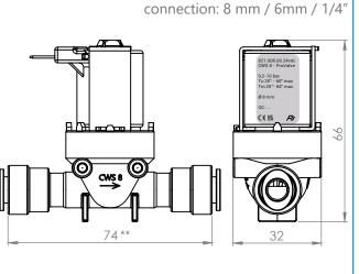
PT Screw connection for plastic body \*\* 10 mm push in length: 78 mm
